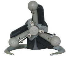
Figure 4: The haptic devices that we used in our evaluation: The 3 DOF Novint Falcon (left) and the 6 DOF Haption Virtuose 6D Desktop (right). The specifications of both force feedback devices show a comparable workspace and a comparable amount of maximum translational force. The 6 DOF device can additionally render torques.
