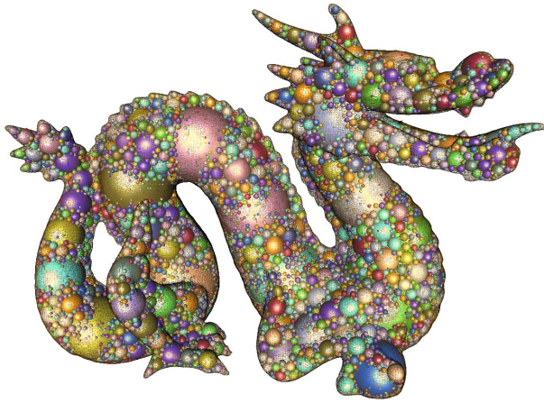
Figure 1: Left: ISTs are based on sphere packings of the object. Right: Such sphere packings enable us to compute an approximation of the penetration volume if the objects overlap.
