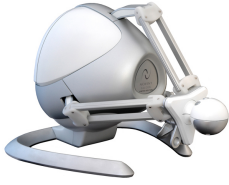
Figure 4: The haptic devices that we used in our evaluation: The 3 DOF Novint Falcon (left) and the 6 DOF Haption Virtuose 6D Desktop (right). The specifications of both force feedback devices show a comparable workspace and a comparable amount of maximum translational force. The 6 DOF device can additionally render torques.
