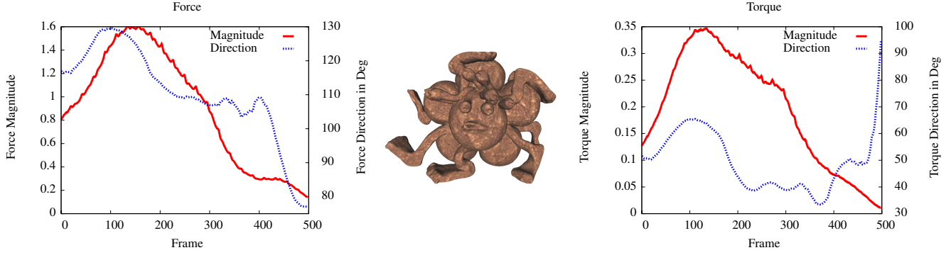
Figure 6: Left: magnitude (red) and direction (blue) of the force arising between two copies of the object shown in the middle, one of which is being moved on a pre-recorded path. Right: torque magnitude (red) and direction (blue) in the same scene.
