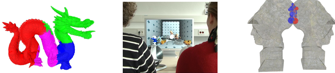
Figure 1: The collision detection in our haptic workspace is based on sphere packings in arbitrary polygonal objects (left). In the accompanying video you can see our haptic workspace set up for two users and four haptic devices. The scene contains more than 20 objects and a total polygon count of 3 millions running on a simple consumer PC with an Intel Core 2 Duo E6700. The haptic devices allow only three DOFs, but the architecture of our workspace supports full six DOF force rendering (middle). The penetration volume defines a novel measure for contact information (right).
